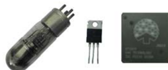
Vacuum Tube, Transistor, an LSI chip
